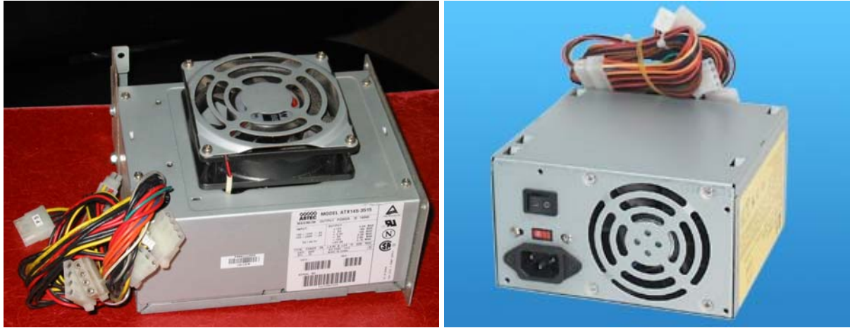
(a) Enclosed Frame Internal Power Supplies
